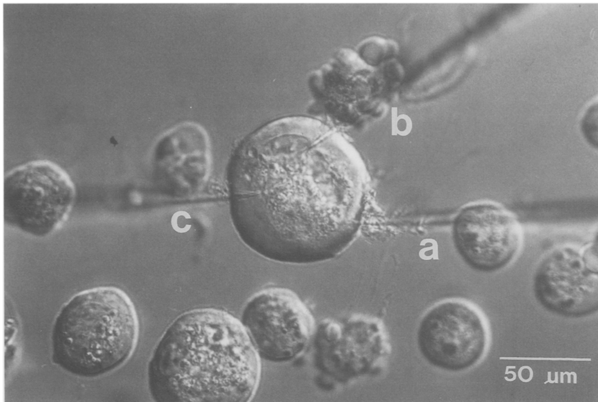
Fig. 1. Simultaneous pH i and plasma membrane K^+ conductance measurements in a fused MDCK cell. (a) current-injecting microelectrode; (b) voltage-sensing microelectrode; (c) pH-sensitive microelectrode
